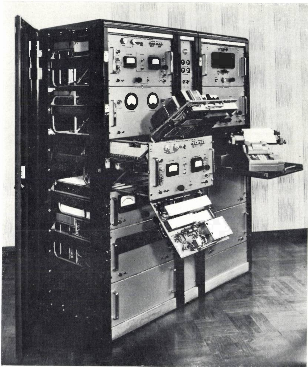
Fig. 10. The correlator. In the three upper left hand units the r.f. signals from the photomultipliers are received, processed and multiplied together. The product signal is processed further in the upper right hand units and the correlation integrals are recorded by the printer shown. The lower units contain the timing and programming units, the E.H.T. supplies for the photomultipliers and the correlator stabilized a.c. supplies.
